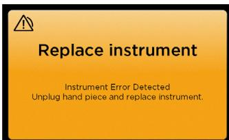
Indicates an internal error with the identification circuitry in the instrument. Special circuitry is installed on certain advanced instruments to identify the device to the generator and tailor the generator's output to the instrument.
