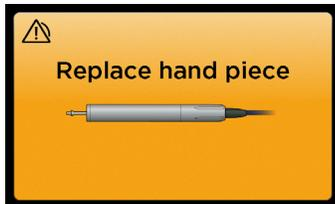
The hand piece has failed to perform the internal diagnostic routines and the generator will not be able to operate the hand piece reliably.
