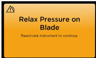
The instrument has been loaded to the point where output has stopped.
